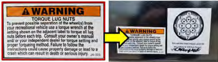
Lug nut torque pattern and warning label
