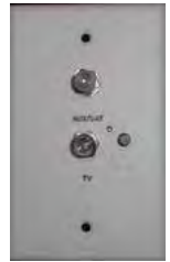
Antenna Power Supply
