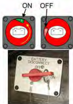
Battery Disconnect Switches Switch appearance may vary by model
