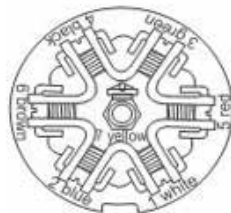
7-way trailer plug car end, rear view
