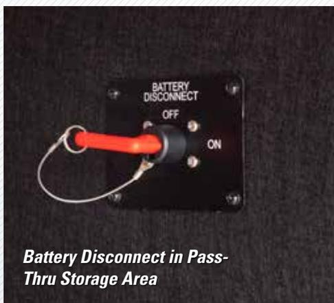
*Battery Disconnect in Pass-Thru Storage Area*
