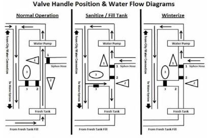
Turning the valve handles in the direction indicated will open or close the valves referenced with each valve handle. The arrows indicate the water flow. Valve #1 (blue handle) is a three way valve. The third position is not used. Valve 2 is a two way valve.
