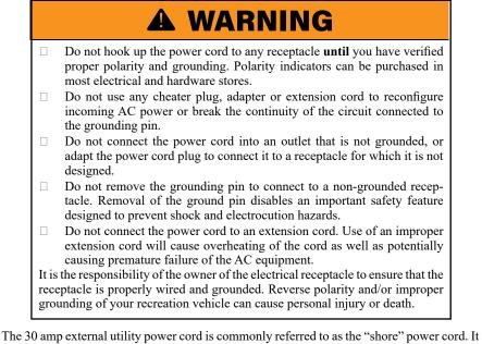
The 30 amp external utility power cord is commonly referred to as the "shore" power cord. It is designed to mate and properly function with 30 amp "shore" power receptacles available at most campgrounds.
