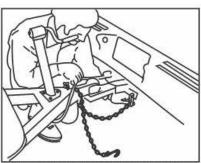
2. Criss-cross left chain and attach to right mounting slot in tow vehicle hitch.
