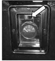
Master / Emergency Shutoff & Fuel Gauge
