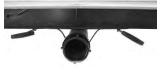
Black/Grey tank drain & valves
