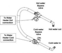
Two Valve Water Heater Bypass Valves shown in NORMAL mode
