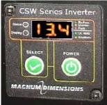
**POWER** button is used to turn the inverter on and off. To turn on the inverter and the LED display press and hold **POWER** for 1 second until you hear a beep.
