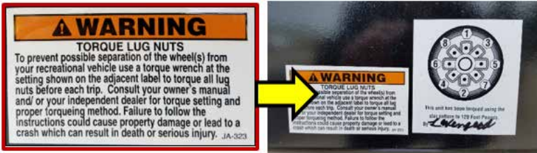
Lug nut torque pattern and warning label
