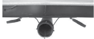
Black/Grey Tank Drain and Valves
