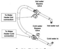
Two Valve Water Heater Bypass Valves shown in NORMAL mode
