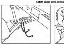
Inspect chains to determine if they are properly attached to trailer frame.
