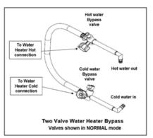
Hot water bypass valve handle (B) should point toward the water heater.
