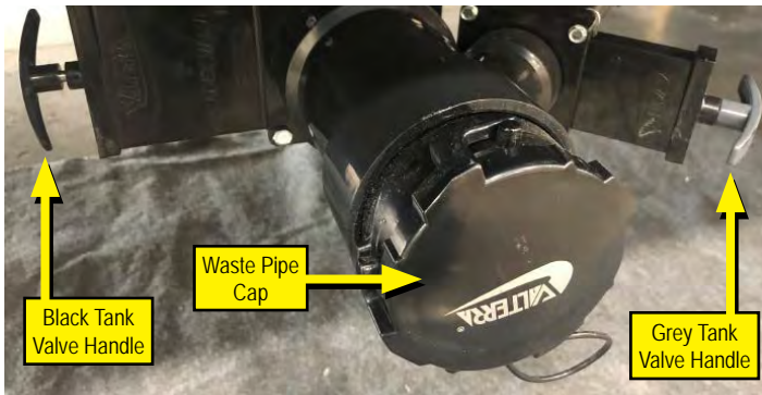
Example of Tank Drain Located Underneath RV
