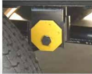
Cam plates shown in neutral position
