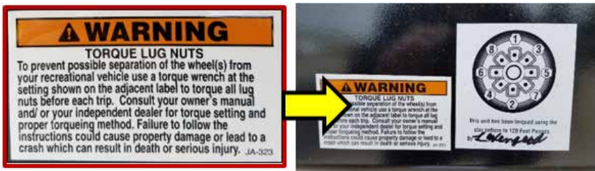
Lug nut torque pattern and warning label
