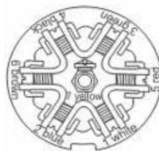
7-way trailer plug car end, rear view
