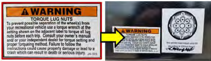
Lug nut torque pattern and warning label
